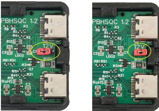
To signal that the PB\_HS\_QC is set to 12V, the LED flashes in a rhythm of 5 seconds after successful connection to the PB.
