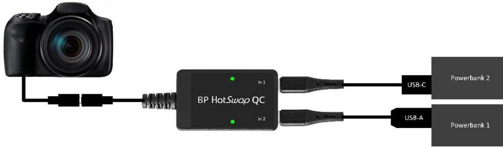
When the PB\_HotSwap\_QC adapter is connected to a QC3.0 or PD powerbank, it requests a voltage of 8.4V from the PB. This is signaled by a slow blinking of the corresponding LED.
