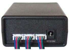
For the connection to the motors, cables with 4-pin XH2.54 connector to 6-pin JST connector can be used, which are offered at a reasonable price for 3D printers.
