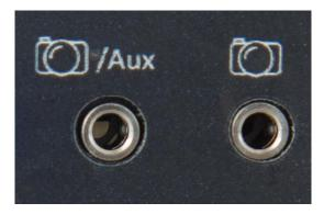
The right socket is the connection for the camera. A 2nd camera can be connected to the left socket or, if necessary, a timer for control if the 2nd port is set as a slave.
